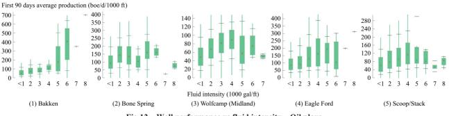
Fig.12 Well performance vs fluid intensity—Oil plays
