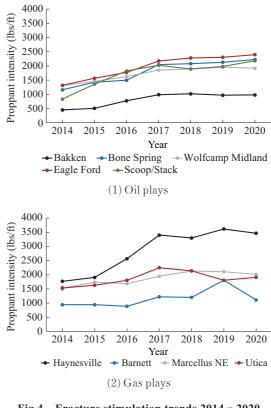
Fig.4 Fracture stimulation trends 2014 – 2020 —Proppant intensity
