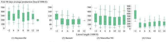
Fig.9 Well performance vs lateral length—Gas plays
