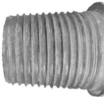
图4 扭矩过小,螺纹被反复研磨变尖
