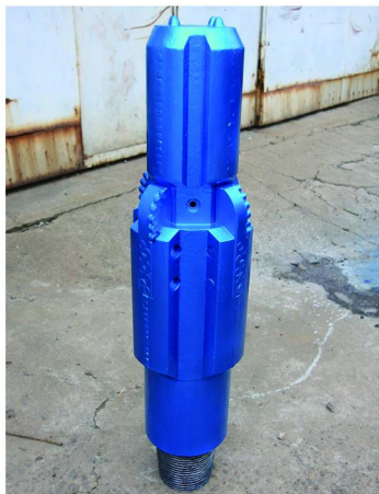
图7 \varnothing 150/202 mm 聚晶金刚石复合片(PDC)扩孔钻头
