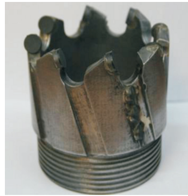
图 5 加长型防斜减振 PDC 复合片钻头外貌 Fig.5 Profile of elongated, stabilized and vibration-reduced PDC bit
