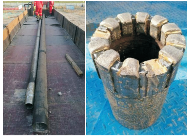
图5 KT194型取心钻具内外管 Fig.5 Inner and outer tubes of KT194 coring tool
