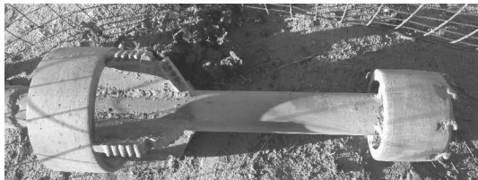
图2 改进后的扩孔钻头 Fig.2 Improved reaming bit
