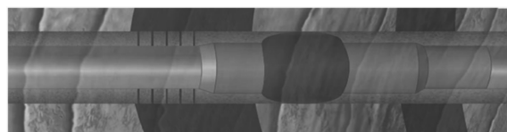
图 3 管外封隔器封隔不同压力、不同流体性质地层 Fig.3 External casing packers isolate the stratum with different pressure and fluid
