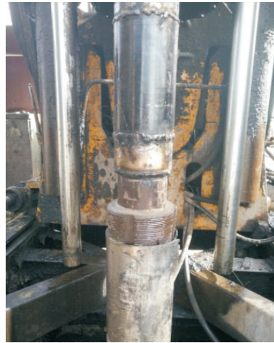
图 6 正丝丝锥打捞套管 Fig.6 Straight thread tap fishing casing
