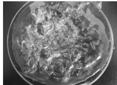
图5 易分散岩心采用一般分散性体系浸泡2 h后的状态 Fig.5 State of easily dispersible cores after soaking for 2 hours in a general dispersive system
