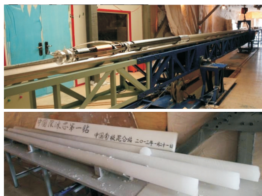
图 3 Dome A 深冰芯钻机及中国深冰芯钻探首季 3 回次冰芯 [5] Fig.3 Dome A deep ice core drill rig and 3 runs of deep ice cores of the first season of Chinese Deep Ice Core Drilling Project in Dome A, Antarctica [5]
