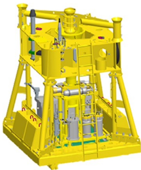
图 3 VOYAGER 钻探船海底基盘外观示意 Fig.3 VOYAGER drill ship subsea base
