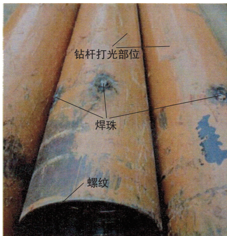
图9 接有KCM装置的钻杆磨损测量情况 Fig.9 Wear of the drill rod with the downhole device KCM
