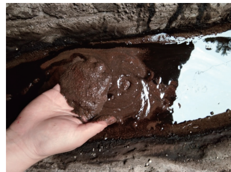
图7 冲洗液携带出来的岩屑 Fig.7 Cuttings carried by the drilling fluid
