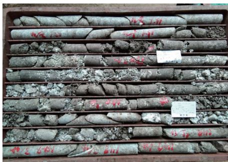
图6 采用成膜防塌无固相冲洗液取出的岩心 Fig.6 Cores taken using film-forming anti-collapse solid-free drilling fluid
