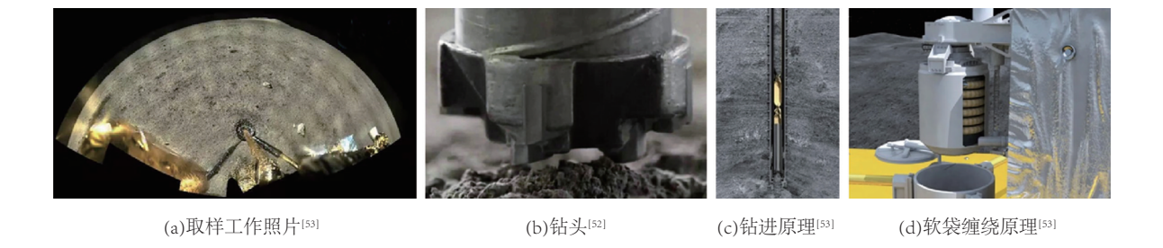
图 20 嫦娥 5 号取样机具 Fig.20 Sample structure of Chang'e-5
