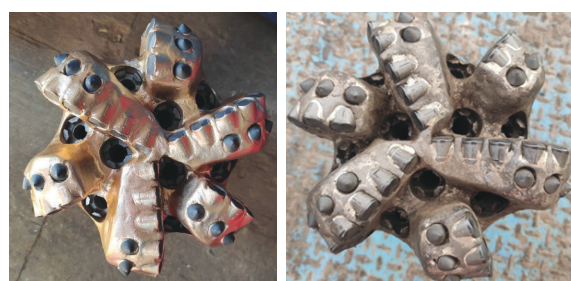
图14 多棱齿+锥形齿钻头 Fig.14 Polygonal tooth + conical tooth bit
