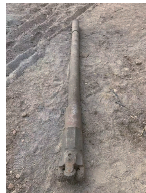
图8 第一回次取心钻进牙轮取心钻头钻具组合 Fig.8 Coring drilling BHA from the first coring-run
