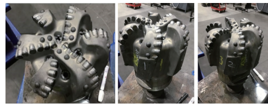
图6 带切深限制钮(DOC control)的PDC钻头 Fig.6 PDC drill bit with depth of cut (DOC) control features
