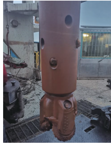
图 9 堵塞的防堵进水短接 Fig.9 Jammed anti-blocking inlet sub
