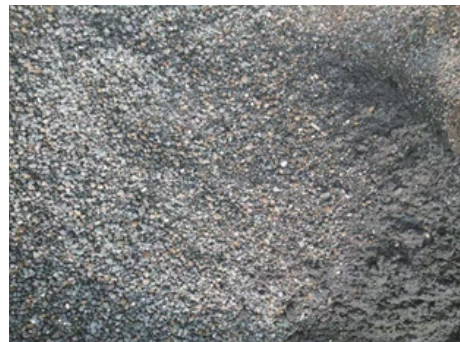
图 11 特别破碎段返出的大量岩屑 Fig.11 Large amount of cuttings returning from the very broken section
