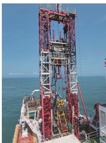
图 5 顶部双驱动联动隔水管钻探取心装置实物 Fig.5 Coring drilling device with the marine top double-drive linkage riser system
