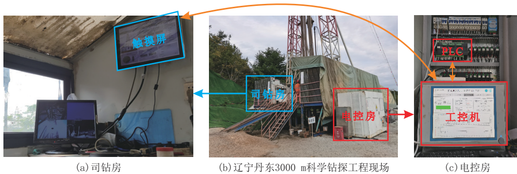
图2 深部地质钻探钻进过程流式大数据分析与预处理系统与工程现场情况 Fig.2 System of streaming big data analysis and pre-processing in deep geological drilling process, and drilling site situation
