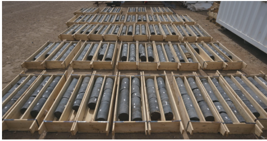
图4 KT216型取心钻具获取的 \text{\O}124\text{ mm} 岩心 Fig.4 \text{\O}124\text{mm} cores obtained by KT216 coring tool
