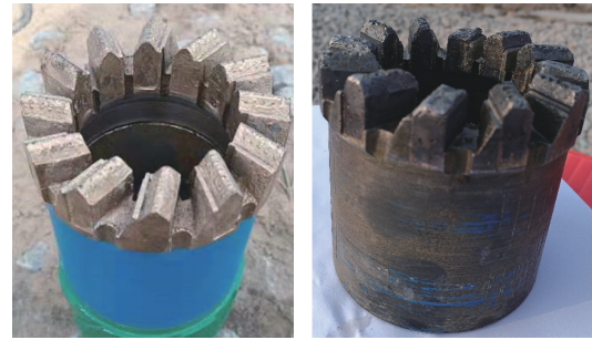
图4 高胎体偏心斜齿孕镶金刚石钻头 Fig.4 High matrix eccentric helical impregnated diamond bit
