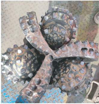
图3 新苏参1井混合钻头使用后照片 Fig.3 Hybrid bit after use in Well XSC-1
