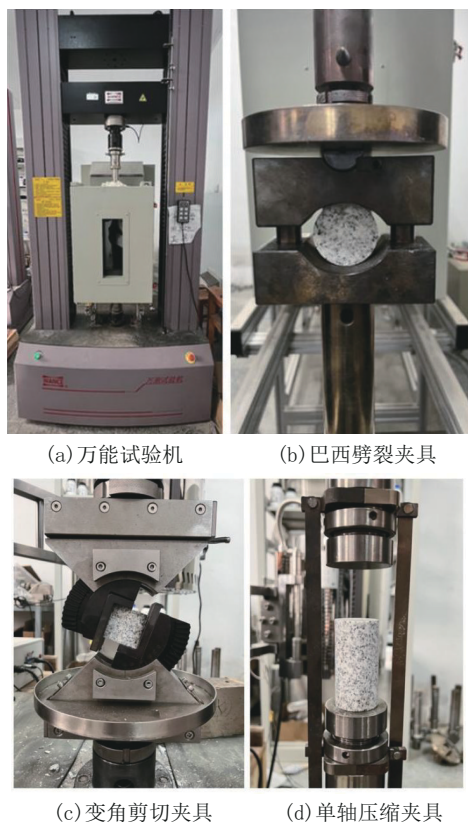
图2 ETM305D型高低温电子万能试验机及试验夹具 Fig.2 ETM305D high low temperature electronic universal testing machine and test fixture
