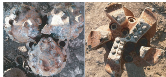
图1 遇砾石磨损严重的钢齿牙轮和常规PDC钻头 Fig.1 Severely wore teal tooth and conventional PDC bit when encountering gravel
