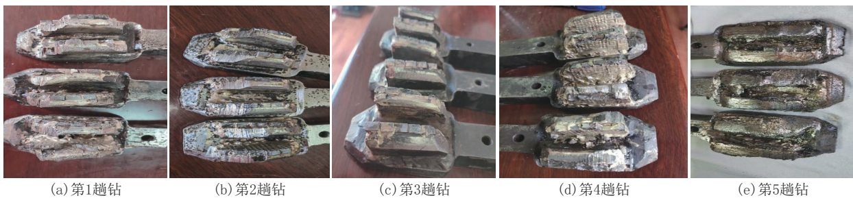
图 6 锻铣工具起出后刀片磨损情况 Fig.6 Wear conditions of the blade after the run
