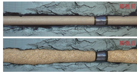
图1 GeoFORM防砂系统原理(来源于贝克休斯公司官网) Fig.1 Schematic diagram of GeoFORM sand control system (from the official website of Baker Hughes)
