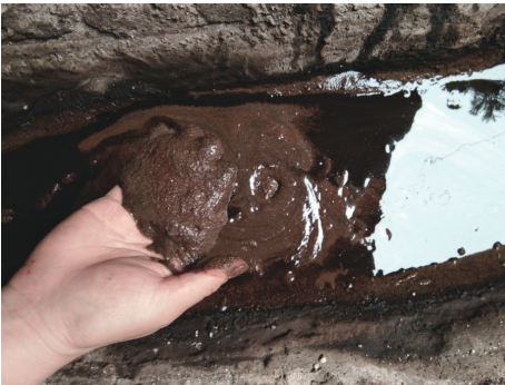
图 6 冲洗液携带出来的岩粉 Fig.6 Rock powder carried out by drilling fluids
