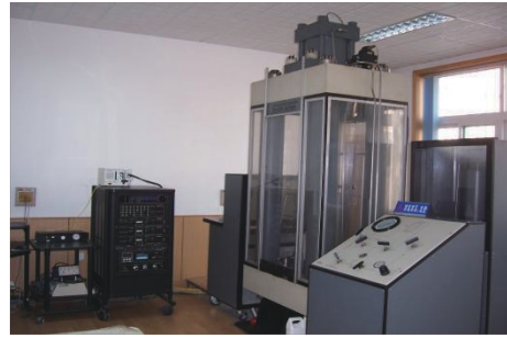
图2 TerraTek岩石力学三轴应力测试系统 Fig.2 TerraTek rock mechanics triaxial stress testing system
