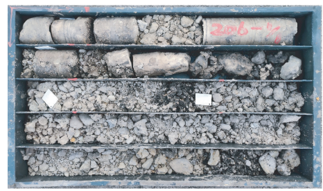
图 5 极松散含砾砂层岩心 Fig.5 Core of extremely loose gravel sand layer
