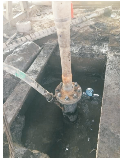
图6 分体式不提钻孔口压水试验孔口装置工作现场 Fig.6 Drilling field of split type wellhead device for water injection test without tripping the drill string
