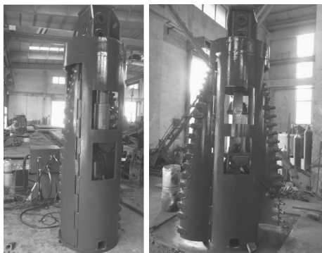
图 2 TGK800/1600 型集土式扩底钻具收翼和扩翼状态 Fig.2 TGK800/1600 soil collecting bell bottom drilling tool in closed/open position
