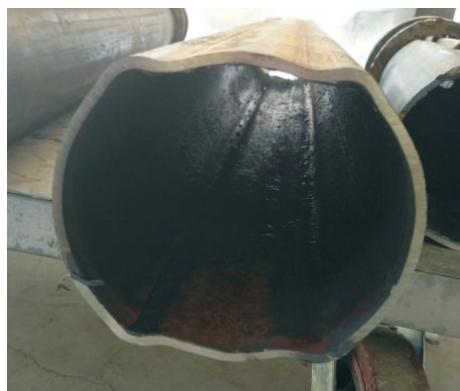
注: TG02 波纹管最大膨胀压力为 13.6 MPa, 膨胀后截面尺寸 D_1=117.8 mm, D_2=137.6 mm, D=131.6 mm
