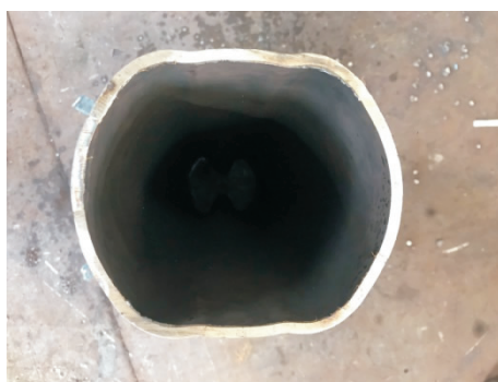
注: TG03 波纹管最大膨胀压力为 12.5 MPa, 膨胀后截面尺寸 D_1=119 mm, D_2=137.8 mm, D=137 mm
