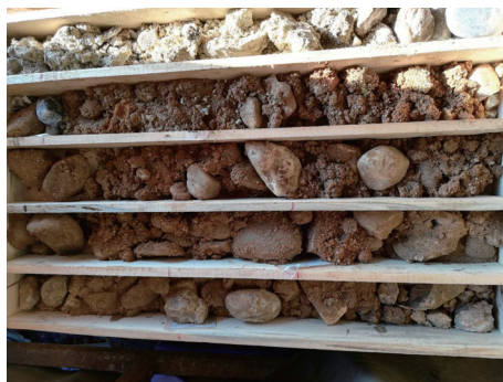
图2 卵砾石层、全风化页岩不稳定复杂地层 Fig.2 Unstable and complex stratum with gravel layers and completely weathered shale
