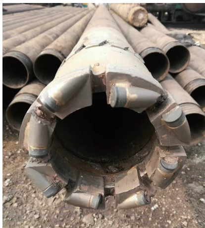
图5 Ø122 mm 绳索取心金刚石复合片钻头 Fig.5 Ø122mm diamond compact coring bit
