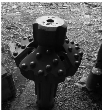
图2 定制的带导向钎头 Fig.2 Customized guiding bit
