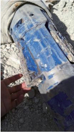
图7 TDX178型锻铣器现场照片 Fig.7 Site photo of the section mill
