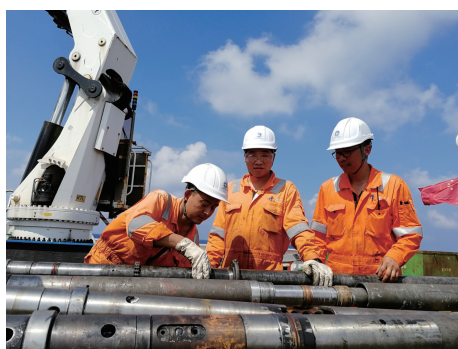
图4 回转式球阀保温保压取样钻具现场调试 Fig. 4 On-site commissioning of the rotary ball valve pressure-temperature core sampler
