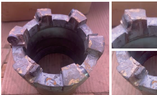
图3 复合片崩齿损坏 Fig.3 PDC broken tooth
