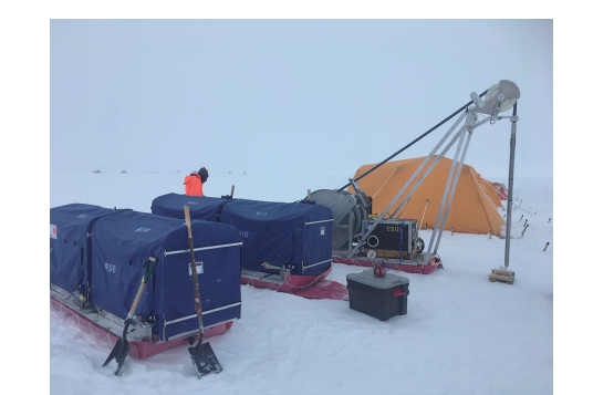
图 15 RAM-2 钻 Fig.15 Rapid Air Movement-2 drill
