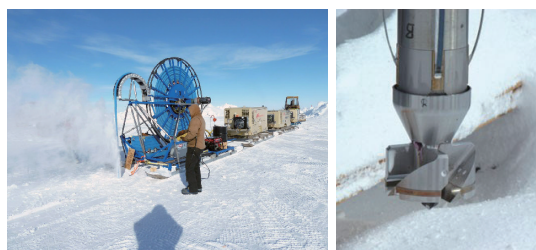
图 14 RAM 钻 Fig.14 Rapid Air Movement drill and drill bit
