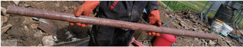
图 19 Ø76.5 mm/Ø49 mm 钻头取出的岩心 Fig.19 Core taken out by Ø76.5mm/Ø49mm drill bit
