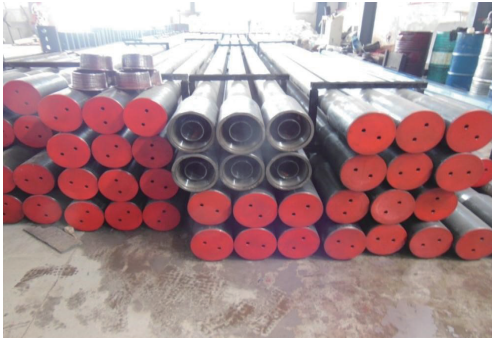
图6 双壁钻杆 Fig.6 Dual wall drill pipe
