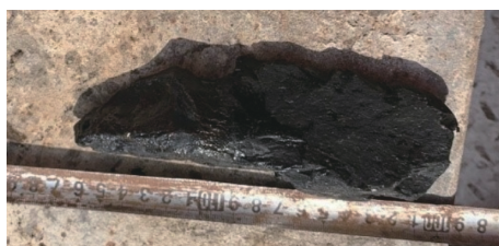
图 16 皖页 1HF 井 17 cm 掉块 Fig.16 17cm falling stone in Well Wanyou-1HF
