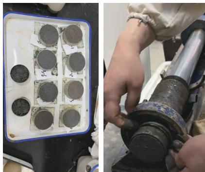
图7 一般物理性质试验样品的制备性表现(砂土) Fig.7 Preparation performance of general physical property of the test samples (sandy soil)
