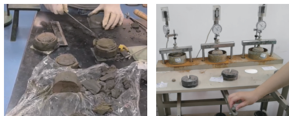
图8 标准固结试验样品的制备性表现 Fig.8 Preparation performance of standard consolidation test samples
