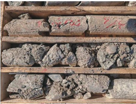
图8 二开井段地层岩心 Fig.8 Formation core of the secondly drilling section
