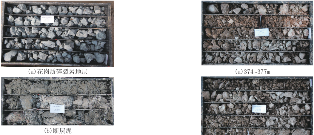
图1 二开孔段花岗质碎裂岩及断层泥岩心 Fig.1 Fault gouge formation encountered in the second spudding
