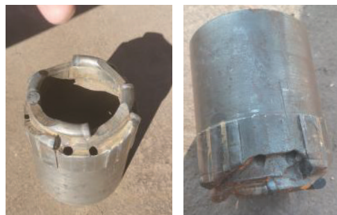
图1 阶梯式侧喷和底喷PDC钻头 Fig.1 Stepped side-injection and bottom-injection PDC bit
