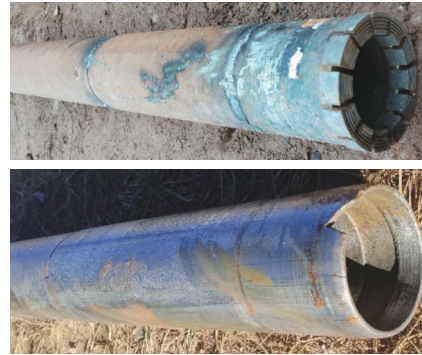
图2 第三次跟管钻进 \varnothing 122 mm 取心钻头入孔前后对比 Fig.2 Comparison before and after the third time using a \varnothing 122 mm coring bit casing while drilling
