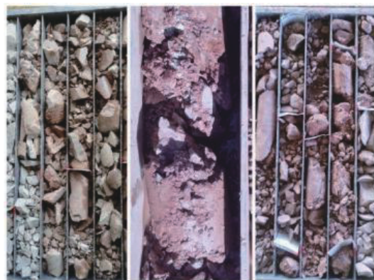
(c)涌水段破碎地层岩心
