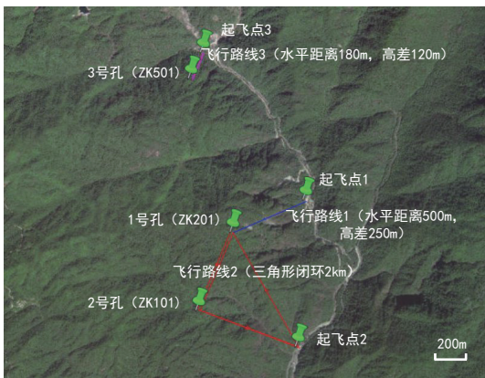
图5 麻江沅工作区无人机吊装飞行路线 Fig.5 Drone lifting flight route in Majiangyuan work area
