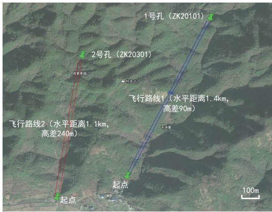
图4 谏家仑工作区无人机吊装飞行路线 Fig.4 Drone lifting flight route in Chenjialun work area
