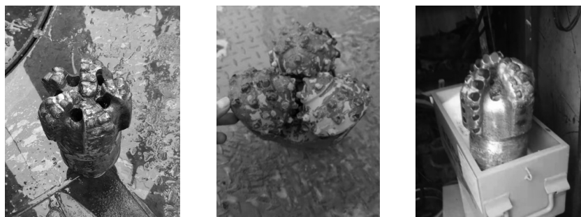
(a)五翼复合片钻头 (b)三牙轮钻头 (c)导向复合片钻头
